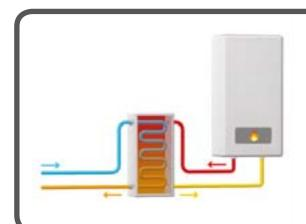
The Lodge range can be fitted with an upgraded electric heater or a heat exchanger, which is an inexpensive, green solution that exploits the heat produced by your facility's heating system or by renewable sources.
