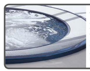
A distinctive feature of the Professional range and Profile Pro is the 15° angled overflow gird around the surface of the hot tub. It collects surface water, which overflows through the grid to a compensation tank. The water is then moved through a filtration system, cleaned and pumped back into the base of the hot tub to be re-used. Thanks to the slant of the grid the water remains at spa deck level even if there is a rocking motion, so they can be installed on yachts and ships.
