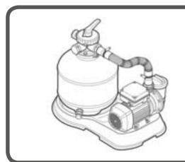
Optional sand filtration gives long standing assurance of hygiene and cleanliness because it traps the impurities in the water. It is easy to remove, must be cleaned on a regular basis and replaced when necessary.
